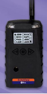
The EchoView Host mini-controller is the cornerstone of RAE Systems' Closed-Loop Wireless Solutions for portable gas monitors. This rugged handheld device can establish a self-contained wireless network with up to eight supported RAE Systems portable monitors and display their readings and alarm status in real time on an easy-to-read screen.
