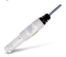
The Rosemount 499AOZ dissolved ozone sensor is ideal for measuring dissolved ozone concentrations in a variety of municipal and industrial applications. The sensor is available with either an integral cable or Variopol (VP6) connector. Variopol cables are sold separately (see Accessories). Rosemount 499AOZ sensors are generally mounted in an off-line low flow cell. Sensors come standard with three replacement membrane assemblies, three O-rings, and a 4 oz (125 mL) bottle of electrolyte.
