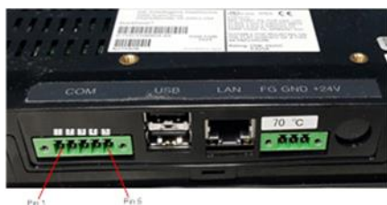
Figure 4.2: IC755CxS06RDx Serial Port COM1 Pin-out
