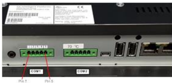
Figure 4.4: C755CxSxxCDx Serial Port COM1 Pin-out
