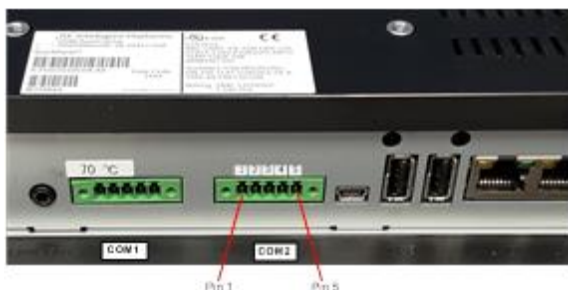
Figure 4.5: C755CxSxxCDx Serial Port COM2 Pin-out
