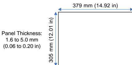
Figure 4.11: IC755CxS15CDx Panel Cutout Dimensions
