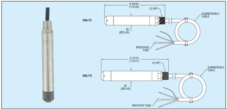
**SBLT2 and SBLTX Submersible Level Transmitters** are manufactured for years of trouble free service in the harshest applications. Both measure the height of liquid above the position in the tank referenced to atmospheric pressure. The transmitters consist of a piezoresistive sensing element, encased in a 316 SS housing. Bullet nose design protects the diaphraem from damage.
