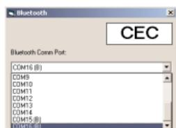
Available Bluetooth serial ports will have a (B) suffix against them in the list. Once you have selected the port, you can test it by performing a test on the MFT1553 and sending the result to the pc/laptop. If the port has been set up successfully you will see a screen similar to the following displayed showing details of the test result:
