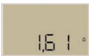
Press the small Red lock button on the MFT1553 Image 91 to cycle round the available result types if applicable. (You will not need to perform this step for rcd results)
