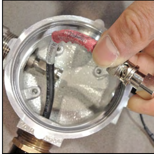
Figure 19: Connecting BNC Plug to the Cable
