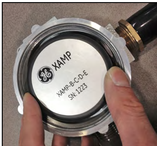
Figure 22: Junction Box Cap
