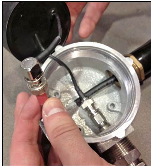
Figure 20: Female Plug to Male BNC Head
