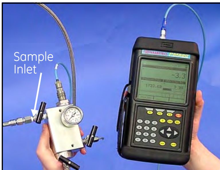
Figure 11: The Sample System and the PM880 AC
