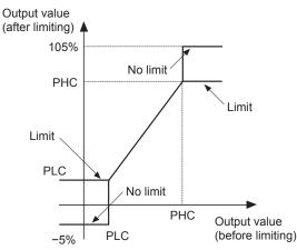
[Setting example] Setting the high and low limit setting to "limit" -
