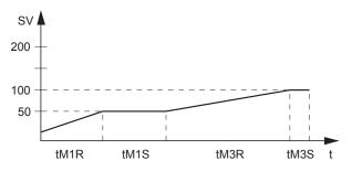
• The SV limit function ([SV-H], [SV-L]) is in effect while ramp soak is running.
