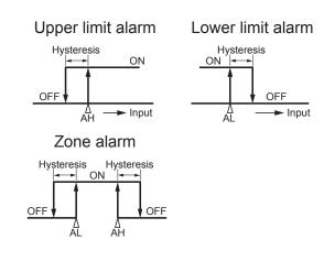
[Setting example] Setting the Alarm 1 hysteresis to 5°C, delay time to 30 seconds —
