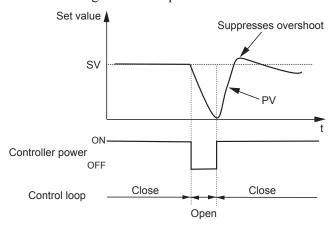
The algorithm used prevents over-integration of the PID calculations even while the control loop is still open. PID2 control can only be used after auto-tuning has been activated and a PID set.
