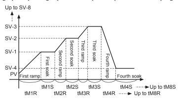
Ramp: the section in which the SV changes toward the target value.
