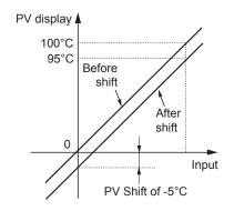
[Setting example] Setting the PV input shift to -5.0°C
