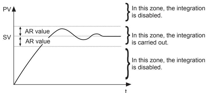
**[Setting example] Changing the anti-reset windup to 500°C**
