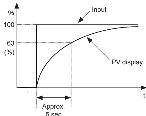
**Note** The factory setting for input filter time constant is 5%.
