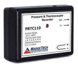
The PRTC110 is a differential pressure and temperature data logger, ideal for use in factory and laboratory applications. The device is available in a 0 to 2inH2O or 0 to 5inH2O model.
