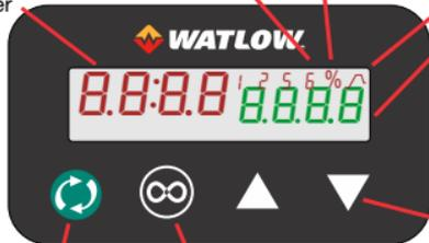
**Right Display:** Home at beginning displays set point (SP). Displays page name when entering pages. Entering into menus displays the parameter name
