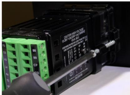
**Figure 3: Tighten the Mounting Screws**
