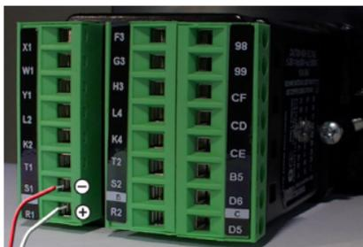
Figure 2: Thermocouple Input Wiring Example
