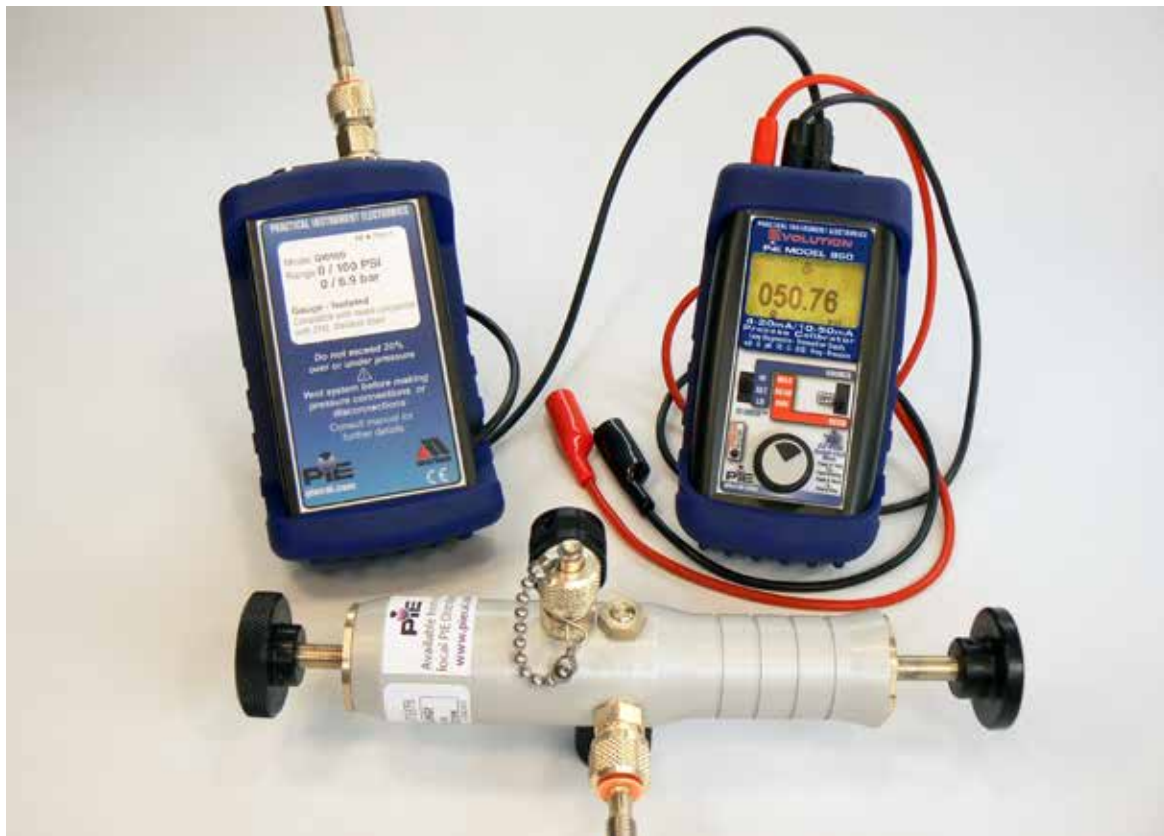
PIE 850 with Pressure Module, Pressure/Vacuum Pump & Hose
