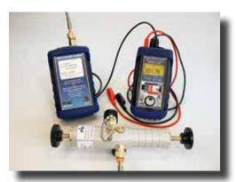
PIE 820-ELITE with Pressure Module, Pressure/Vacuum Pump & Hose
