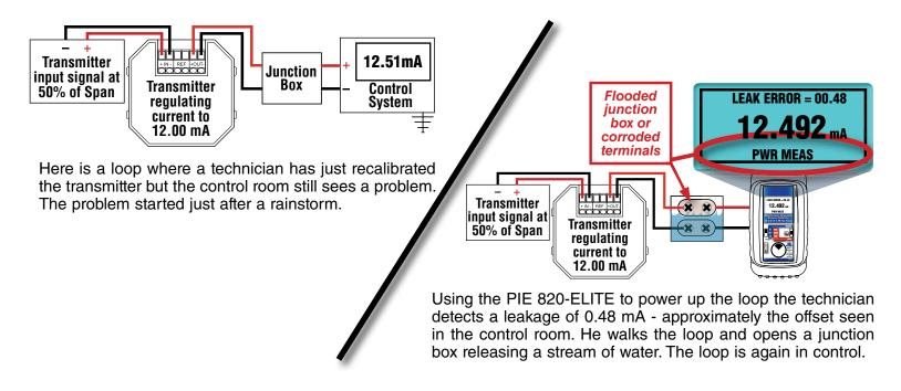
Why buy a PIE calibrator with loop diagnostics Undiagnosed loop problems often cause calibration errors which can lead to dangerous operating conditions or catastrophic results. The PIE 820-ELITE is the *only single display multifunction calibrator* that can detect and indicate these problems due to the patented troubleshooting features.
