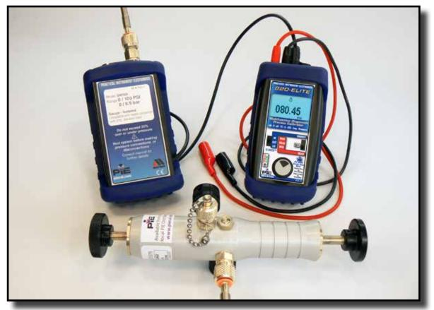
PIE 820-ELITE with Pressure Module, Pressure/Vacuum Pump & Hose
