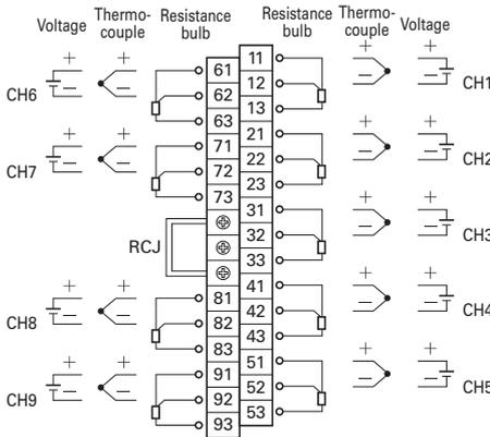
(Note) For current input, connect an optional shunt resistance to a voltage input terminal
