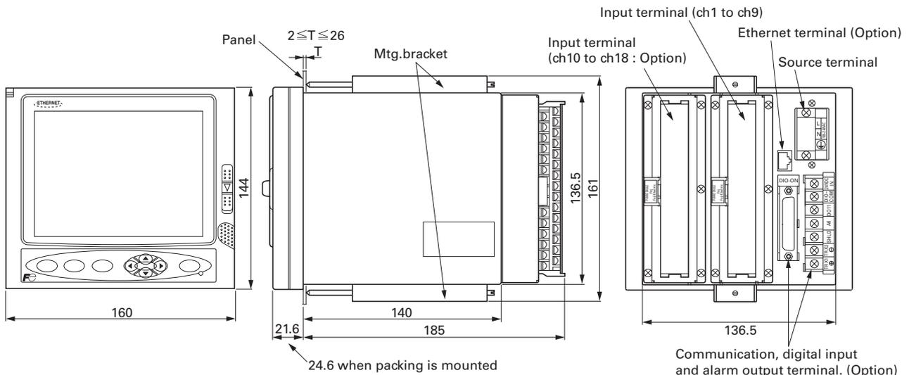
(Note) When placing the main unit on another instrument or on the floor, allow a space of 100mm or more between the unit and instrument or the floor.
