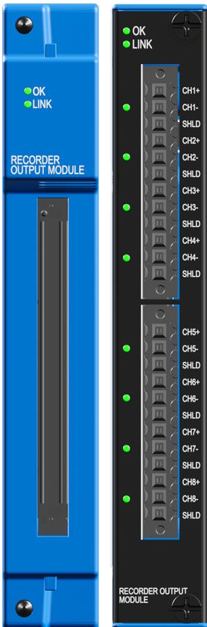
The recorder output module is a 8-channel single slot width module that provides an analog output signal based on a processed measurement from any of the proportional measurements within the system. The output of the recorder output channel is proportional to the associated measurement value within the measurement's full scale range.
