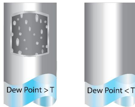
**Figure 30** Condensation in Sample Tubing
