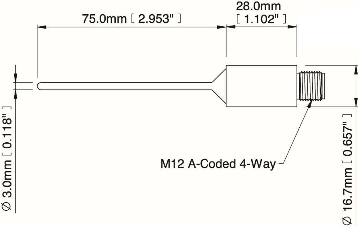
\*Weld burr may extend from 1mm from collar to towards tip of probe.
