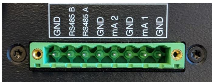
*Figure 11 RS485 & Analog output connector*
