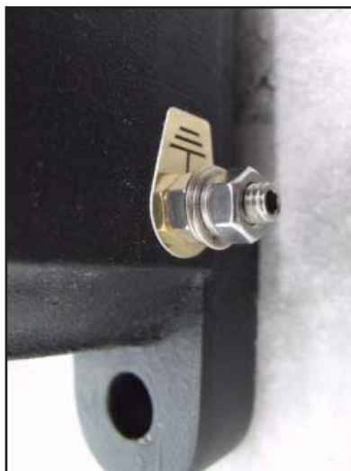
Figure 5 Earthing Stud And Nut Washer Assembly
