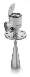
Designed for basic liquid applications, this market entry 24 GHz 2-wire FMCW radar transmitter provides accurate readings even in fast moving processes, in closed tanks or in the open air like rivers or dams. Its proven PP Drop antenna is insensitive to condensation.
