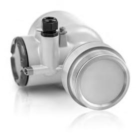
Accurate continuous level measurement of fine powders has to deal with a series of issues like dust, low-reflective media, build-up and uneven surfaces. The specific algorithms and high signal dynamics of this 80 GHz FMCW radar transmitter are the key to provide reliable and accurate readings despite these difficult conditions. Thanks to the small beam angle of the flush-mounted Lens antenna, this powerful device handles high and narrow silos even in the presence of internal obstructions.
