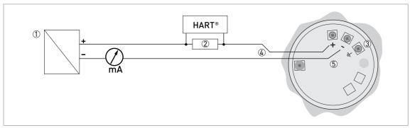
Figure 4-2: Electrical connections for non-Ex devices
