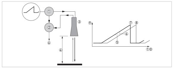
Figure 1-1: Measuring principle of FMCW radar
