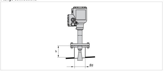
Figure 3-6: Flange connections
