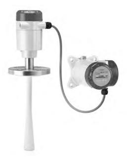
This 10 GHz 2-wire FMCW radar level transmitter measures distance, level, volume, mass and flow rate of liquids and pastes. It is ideal for corrosive products with its PP or PTFE antenna options. It features unique PP and PTFE antennas for aggressive products. The device is able to measure distances up 30 m / 98.4 ft in process conditions up to +250°C / +482°F and 40 barg / 580 psig.
