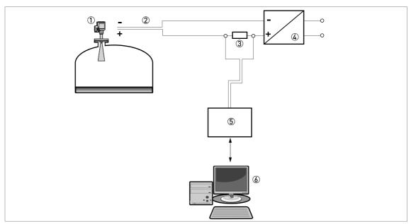
Figure 4-3: Point-to-point connection (non-Ex)
