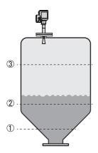
A strapping table function is available in the configuration menu for volume or mass measurement. Up to 50 volume (mass) values can be related to level values. For example:
