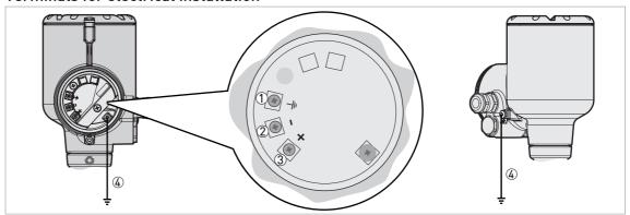
Figure 4-1: Terminals for electrical installation
