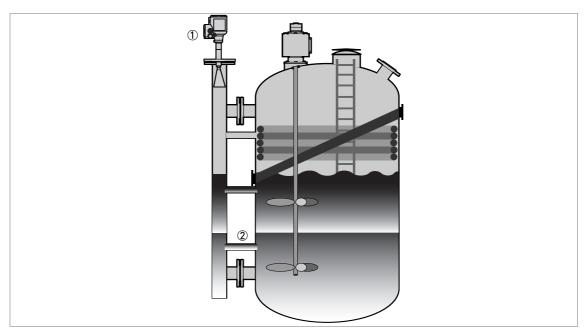
Figure 3-13: Installation recommendations for bypass chambers that contain more than one liquid
