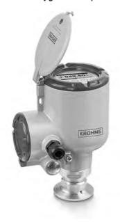
This 80 GHz FMCW radar transmitter for hygienic liquid applications in the pharmaceutical, food and beverage industries is CIP-SIP suitable and offers a large choice of hygienic process connections: Tri-Clamp®, Tuchenhagen VARIVENT®, SMS, DIN 11851, DIN 11864-1 Form A, NEUMO BioControl®.
