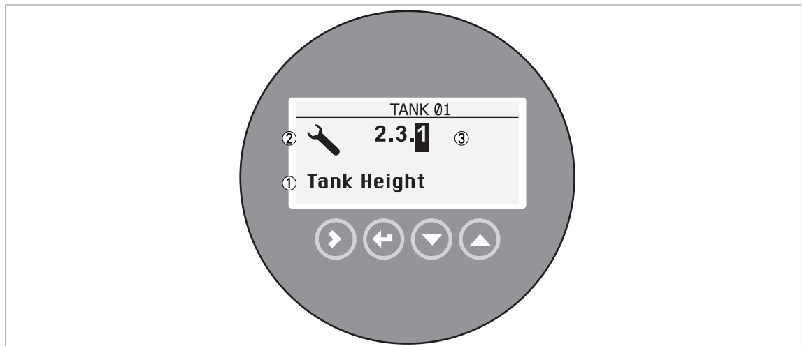
Figure 6-1: Local display screen layout in configuration mode
