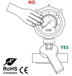
After installation the vent plug can be cut to relieve internal pressure changes in the gauge case that otherwise would have been induced by environmental changes in pressure and/or temperature. Without being vented this change in internal pressure could adversely affect the accuracy of the gauge. If liquid filled, only open vent plugs when the plug is oriented in the vertical position.
