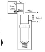
3 WIRE WIRING DIAGRAM EXAMPLE
