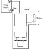
3 WIRE WIRING **DIAGRAM EXAMPLE**
