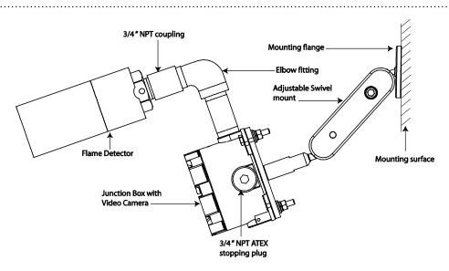
Note: It is recommended that a sunshade kit be fitted on the video camera enclosure (junction box) if FlameWatch II is going to be continually exposed to direct sunlight, which may result in temperatures beyond 75°C.
