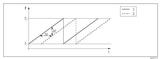
FMCW principle: Results of the frequency modulation
