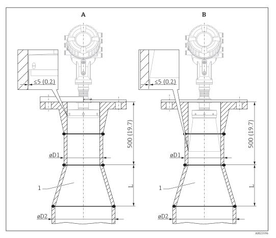
Installation of NMR84 in stilling wells with a larger diameter
