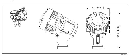
I1 Dimensions of the electronics housing; unit of measurement: mm (in); adapters for cable entries are not taken into account in this drawing.
