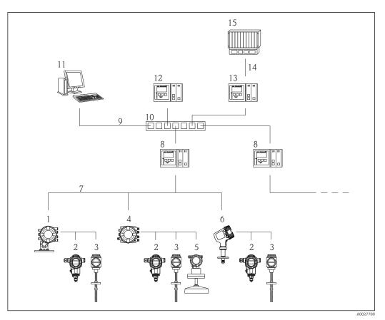
Integration of tank gauging devices into an inventory management system (typical example)
