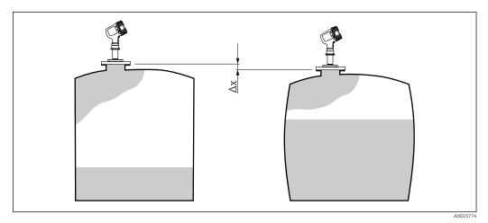
■ 18 Movement ∆x of the Gauge Reference Height due to the bulging of the tank shell caused by hydrostatic pressure
