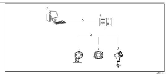
🖻 16 Remote operation of Tank Gauging devices
