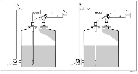
Integration of tank sensors with Micropilot (Example)
