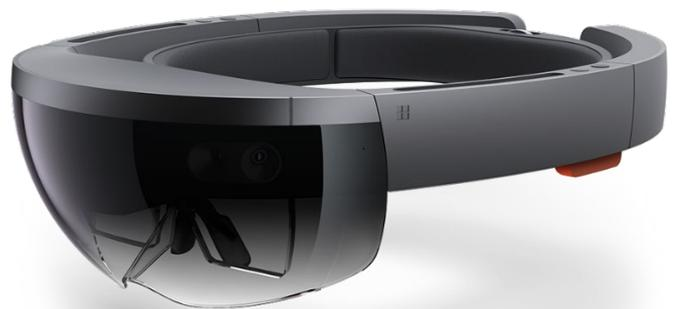
environmental analysis. An additional camera can detect depth in order to recreate the surrounding environment, while a 2-megapixel HD camera is used for taking pictures and shooting video. Vocal commands are captured by four microphones embedded in the display. According to Microsoft, HoloLens can gather terabytes of data from sensors and process it in real time. The device senses where the operator is looking, interprets his/her gestures and understands his/her vocal commands.
