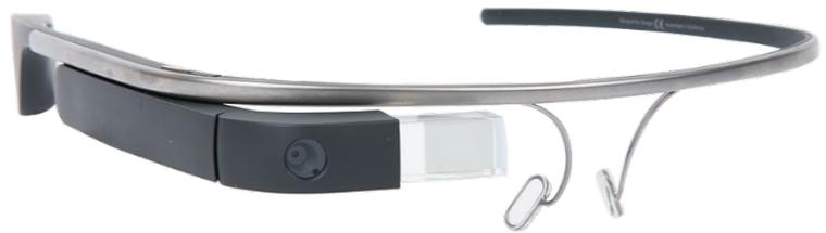
applications. This device offers several additional functions thanks to the integration of camera, inertia sensors, speakers and microphone, used for controlling Google Glass via vocal commands. It constitutes a real stand-alone wearable device, in that the application can be displayed directly on the glass and does not need any other external device. The product is still being tested, as Google is making hardware changes based on the user feedback.
