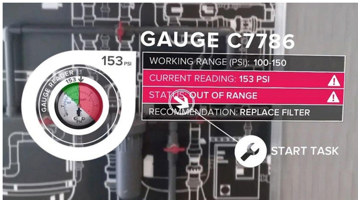
*Example of Augmented Reality application where the display overlays dynamic data from the supervision system and the data server on the surrounding environment.*
