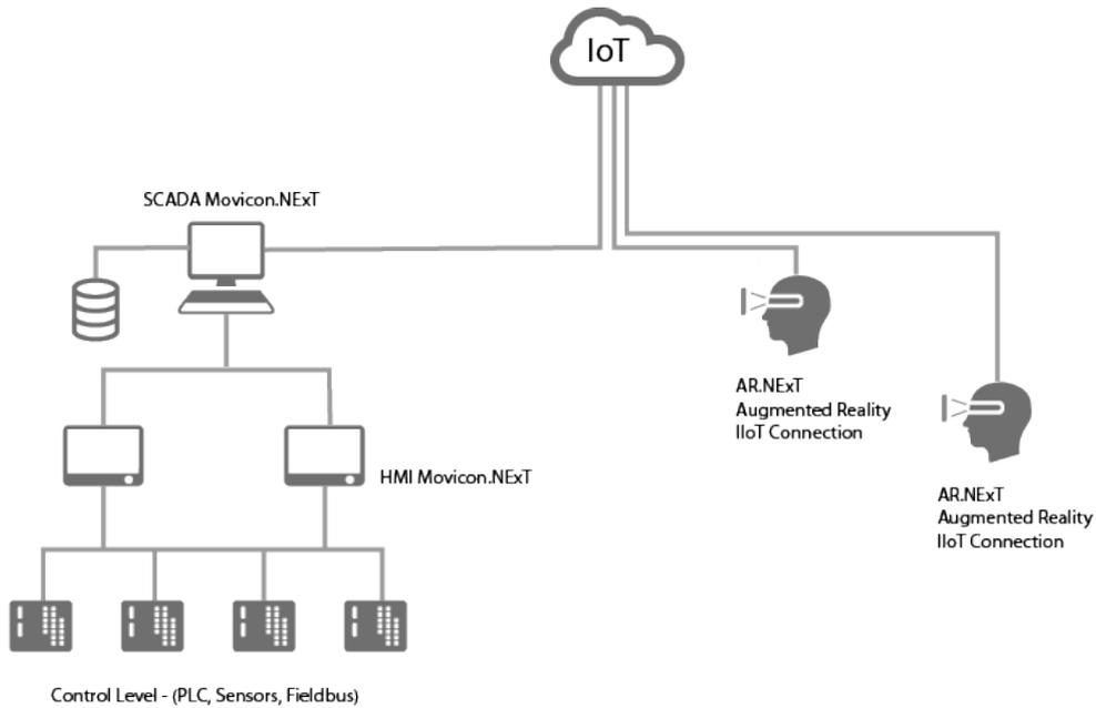
*Example with Augmented Reality devices (for HoloLens only)
