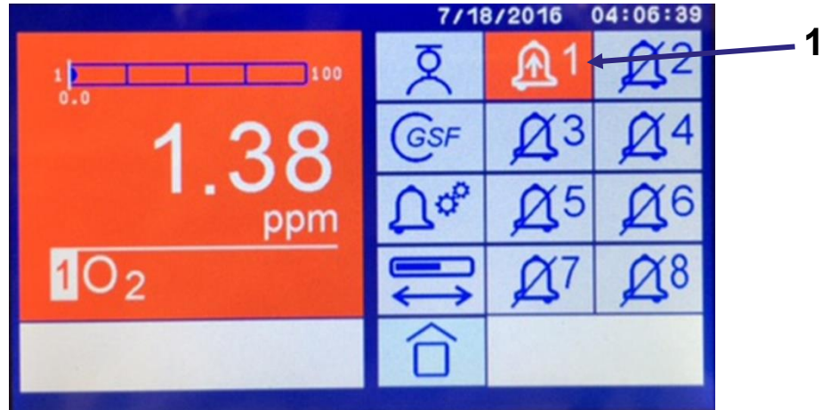
Figure 5-23: Alarms screen showing triggered alarm
