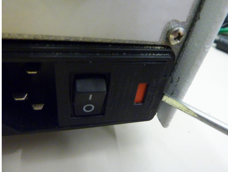
Figure 10-1: Open the fuse panel
