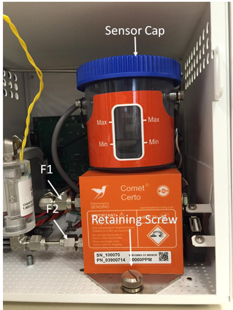
Figure 5-1: Disconnect the gas fittings
