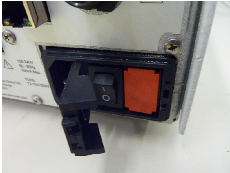
Figure 10-2: Fuse panel opened
