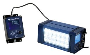
The illumiNova Remote Controller allows for safe operation (up to 100 feet) away from an illumiNova that is installed in an inaccessible location. A 25 foot Cat 5E interconnect/power cable is included. Standard Cat 5E Ethernet\* patch cables with RJ45 connectors, up to 100 feet long, can be used if longer distances are needed.
