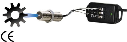
**M-190 (Magnetic Sensor):** Most popular sensor for use with 60 tooth 20 pitch gears. Sensor mounts within 0.005 inches (0.127mm) of a minimum 0.1 inch (2.5mm) target. Requires no power from the display module and self-generates an AC signal.
