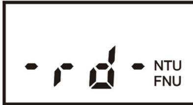
The instrument will display moving dashes on the screen for 6-7 seconds prior to displaying a value. This will occur prior to taking a reading & prior to indexing. No keypad presses will operate during this time.
