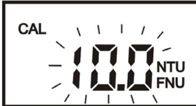
5. Insert the 10.0 NTU standard into the sample well and press down until the cuvette snaps fully into the instrument. Align the indexing ring with the arrow on the instrument (see section 4.2 if the standard is not already indexed).
