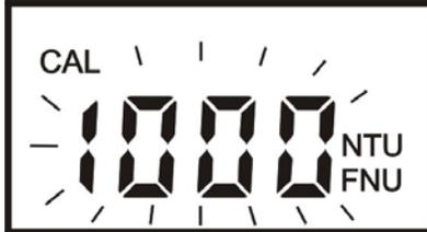
2. Insert the 1000 NTU standard into the sample well and press down until the cuvette snaps fully into the instrument. Align the indexing ring with the arrow on the instrument (see section 4.2 if the standard is not already indexed).
