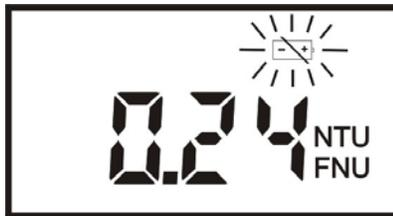
A solid battery icon on the display indicates that power level is too low and the readings may be out of specification. Under this condition, the batteries should be replaced as soon as possible to ensure that the instrument will continue to function properly. If the batteries get too low to perform, the instrument will turn off & the instrument may not turn on until the batteries have been replaced. See section 6.2 for more information
