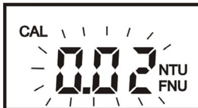
8. Insert the 0.02 NTU standard into the sample well and press down until the cuvette snaps fully into the instrument. Align the indexing ring with the arrow on the instrument (see section 4.2 if the standard is not already indexed).
