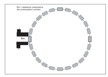
Figure 21: Commutator with 24 Coils in Series
