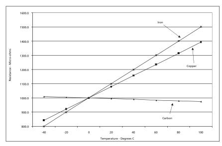
Figure 18: Temperature-Resistance Curves for Iron, Copper and Carbon
