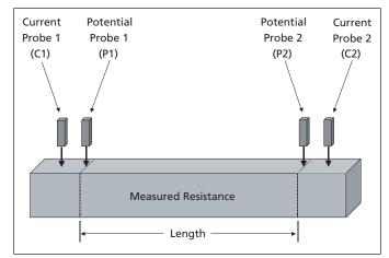
Figure 11: Simplified Example of a 4-Wire Measurement
