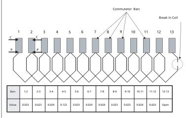
Figure 20: Testing a Lap Winding
