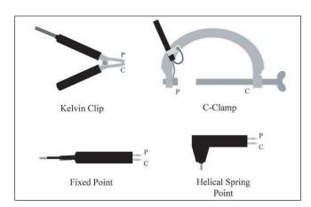
Figure 17: Basic Styles of Probes
