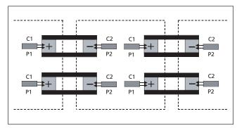
Figure 5: Parallel Straps on a Large Battery Complex
