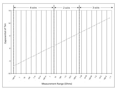
Figure 10: Selection of Optimum Measuring Technique
