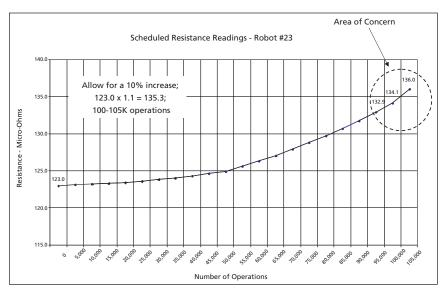
Figure 15: Trending Analysis of Low Resistance Readings
