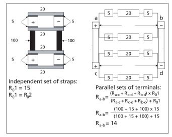
Figure 25: Parallel Strap Resistance Target
