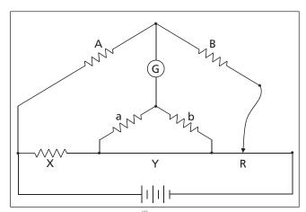
Figure 27: Kelvin Bridge Circuit<sup>viii</sup>
