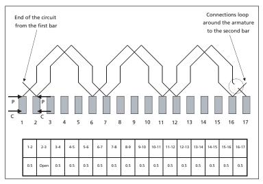
Figure 22: Testing a Wave Winding
