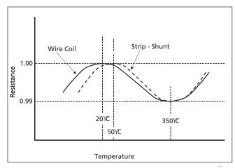
Figure 1: Qualitative Resistance-Temperature Curve for Manganin<sup>iii</sup>
