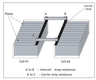
Figure 6: Measuring Carrier Strip Resistance
