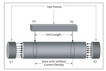
Figure 7: Testing Graphite Slugs for Uniform Density (ohms/inch)
