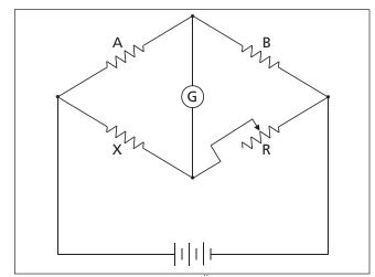
Figure 26: Wheatstone Bridge circuit<sup>VII</sup>
