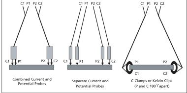
Figure 14: Probe/Lead Configurations
