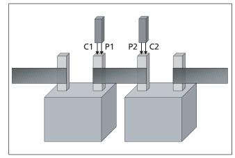
Figure 4: Single Strap with Two Contact Surfaces
