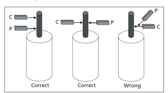
Figure 16: Correct and Incorrect Probe Placements
