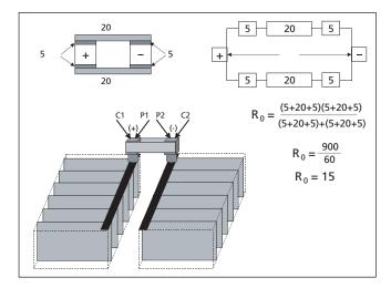
Figure 24: Single Strap Resistance Target
