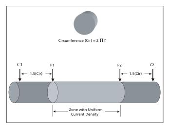
Figure 13: ASTM Standard B193-65
