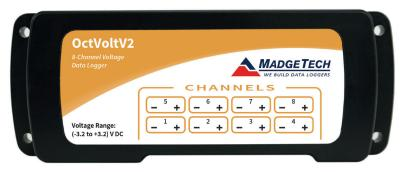
The OctVoltV2 is an 8-channel, battery powered, DC voltage data logger with reading rate up to 4 Hz reading rate. It can measure and record up to 174,592 readings per channel. To maximize memory capacity, users can enable or disable channels. For easy identification, each channel can be named with up to a ten digit title.
