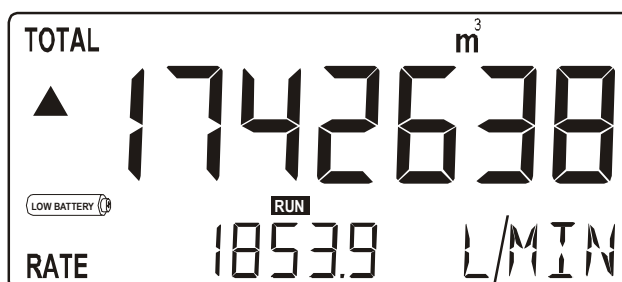
Fig. 4: Example of low-battery alarm.
