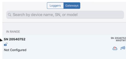
If the gateway does not appear, make sure it is completely powered up as described in step 3 and within range of your phone or tablet.
