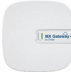
For wall mounting, position the gateway facing the coverage area with the logo oriented as shown
