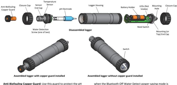
Anti-Biotouling Copper Guard: Use this guard to protect the pH electrode when deploying the logger in water prone to biofouling (see *Deploying and Mounting the Logger*).
