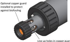
Line up holes in copper guard with holes in sensor end cap and pH electrode
