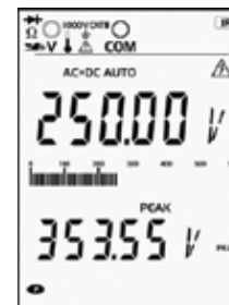
PEAK Mode Example of screen showing Peak+ value
