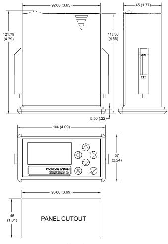
Dimensions are in millimeters (inches). Weight = 0.55lb (0.25kg).
