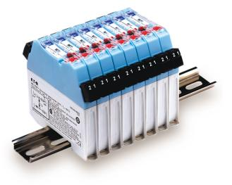
**MTL7700 active modules** are protected with an electronic fuse for the majority of applications. The MTL7798 active fused, power feed module can protect up to 40 other modules using the bussed power facility and provides a clear indication of a trip condition via a red LED.
