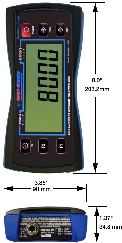
Figure 7-1. Mechanical Dimensions
