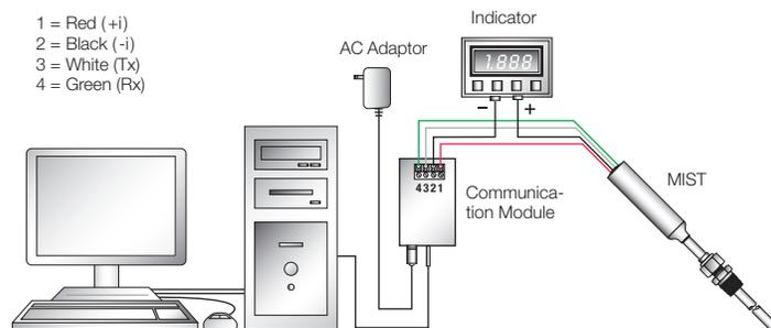
The MIST Temperature Sensor™ connected to a PC via the MIST PKIT-1
