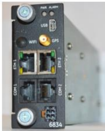
Figure 6-3 Platform Manager Module
