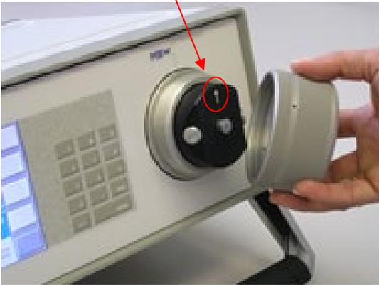
1. Install the optical assembly, taking note of guide pin (s) and alignment indication
