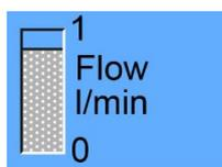
Using the flow meter indication on the 973 status line, observe and set the flow rate in the range 0.5 to 2 LPM.
