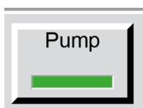
As the 973's measuring head is internal, to obtain a representative sample, flow through the measuring head is required from the internal sample pump. Press the **Pump** button to generate gas flow. Pump power can be varied, see chapter 5.4.8 'Sample Pump' on page 36.
