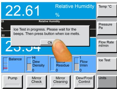
When you observe the phase transition on the mirror, press the **Ok** button. The mirror temperature is measured at that moment and a dialog box appears with the test results.
