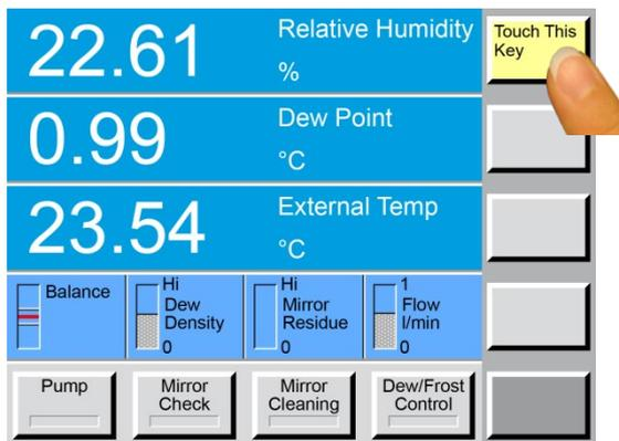
With the tip of your finger, press the center of the yellow highlighted key. After a successful detection you will hear a click and the yellow Key switches position.
