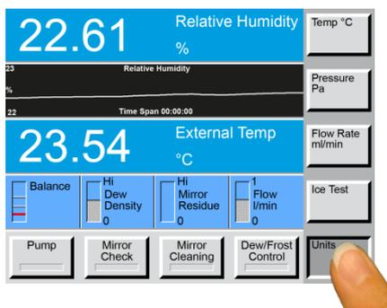
Press the menu selection key on the lower right to select the **Diagnostic Functions** menu. Then press the **Ice Test** button.
