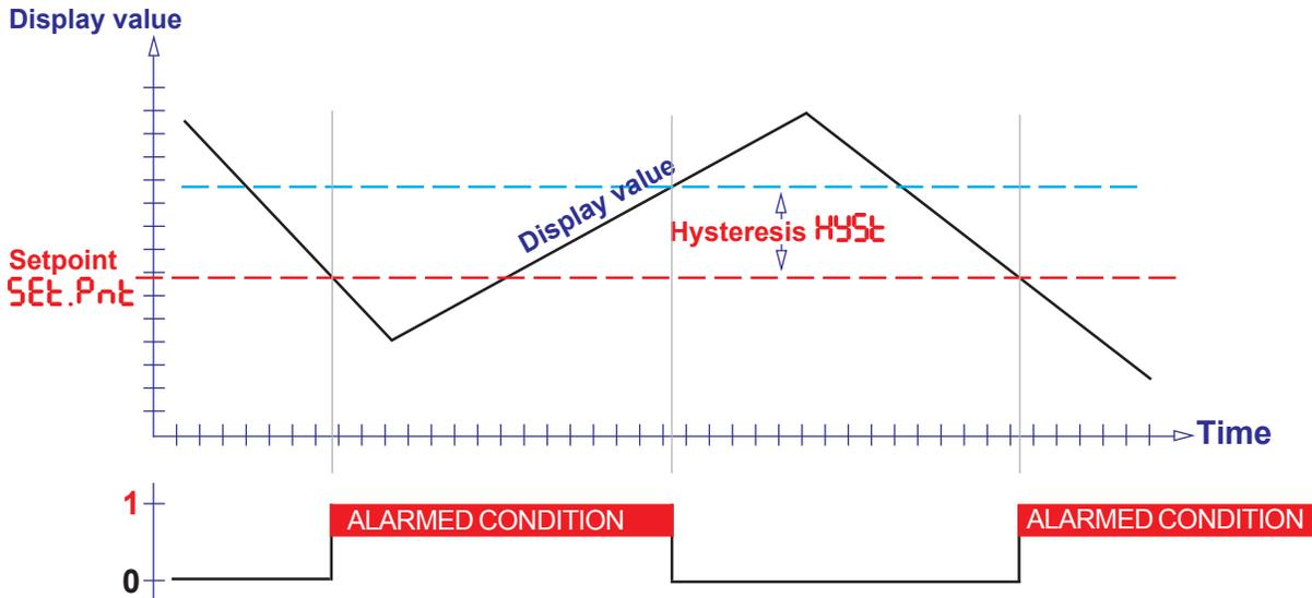
The Setpoint can be placed anywhere you like, in the range **-999999** to **+999999** and will include a decimal point in the appropriate position if you have set your display range to have a decimal point.
