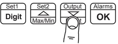
**Each press of the DOWN arrow, or UP arrow will alternate between showing **Adv.** or **EASY****
