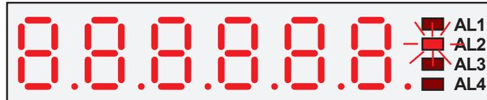
The display will show (in dim numerals) the existing setpoint level for that alarm, or it will show **OFF** if that alarm has not yet been given a mode.
