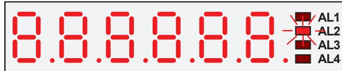
The display will show (in dim numerals) the existing setpoint level for that alarm, or it will show **OFF** if that alarm has not yet been given a mode.
