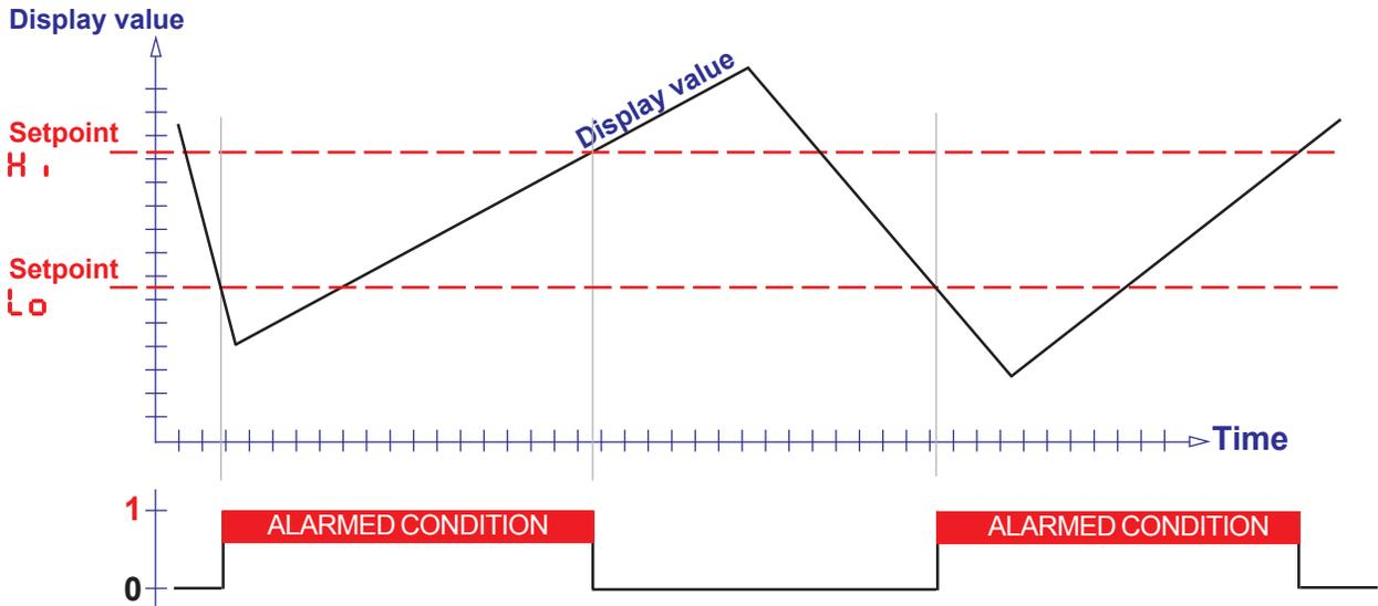
The Setpoints can be placed anywhere you like, in the range **-999999** to **+999999** and will include a decimal point in the appropriate position if you have set your display range to have a decimal point.
