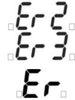
'Er2' is displayed when the thermometer is exposed to rapid changes in the ambient temperature. 'Er3' is displayed when the ambient temperature exceeds 0°C(32°F) or +50°C (122°F). The thermometer should be allowed plenty of time (minimum 30 minutes) to stabilize to the working/room temperature.
