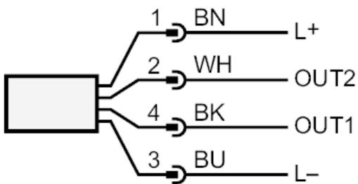
OUT1: switching output or IO-Link
