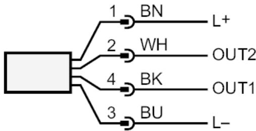
OUT1: switching output or IO-Link
