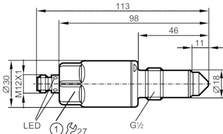
1 Tightening torque 20...25 Nm
