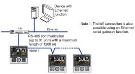
An Ethernet connection is also possible using controllers with an RS-485 communication function and an Ethernet/RS-485 converter (Yokogawa VJET is recommended).
