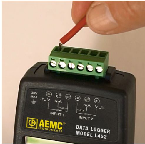
Figure 24. Inserting a lead into the terminal strip
