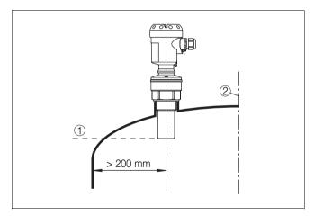
Fig. 5: Mounting on dished vessel tops
