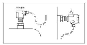
Fig. 2: Measures against moisture penetration
