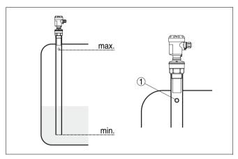
Fig. 14: Standpipe in a tank 1 Vent hole ø 5 ... 10 mm
