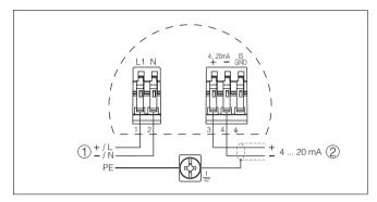
Fig. 19: Wiring plan, double chamber housing
