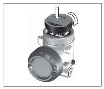
Fig. 20: Installation of the indicating/adjustment module
