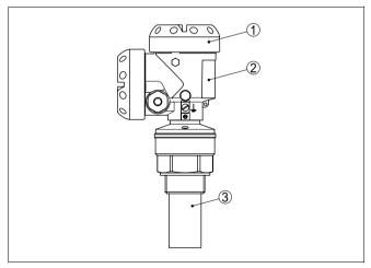
Fig. 1: OPTISOUND 3010 C with Alu double chamber housing
