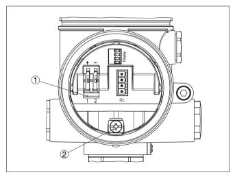
Fig. 18: Connection compartment, double chamber housing
