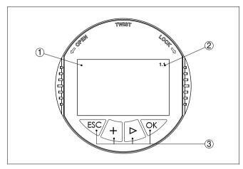
Fig. 21: Indicating and adjustment elements
