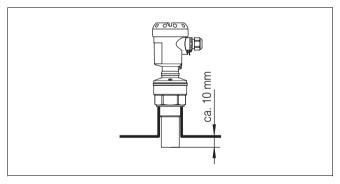
Fig. 7: Recommended socket mounting
