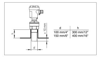
Fig. 8: Deviating socket dimensions
