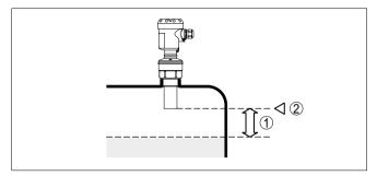
Fig. 3: Min. distance to the max. level
